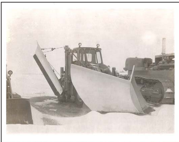
Photo of an old V-plow and wing mounted on a loader. date taken unknown, came from Wayne Cramer's old files.
