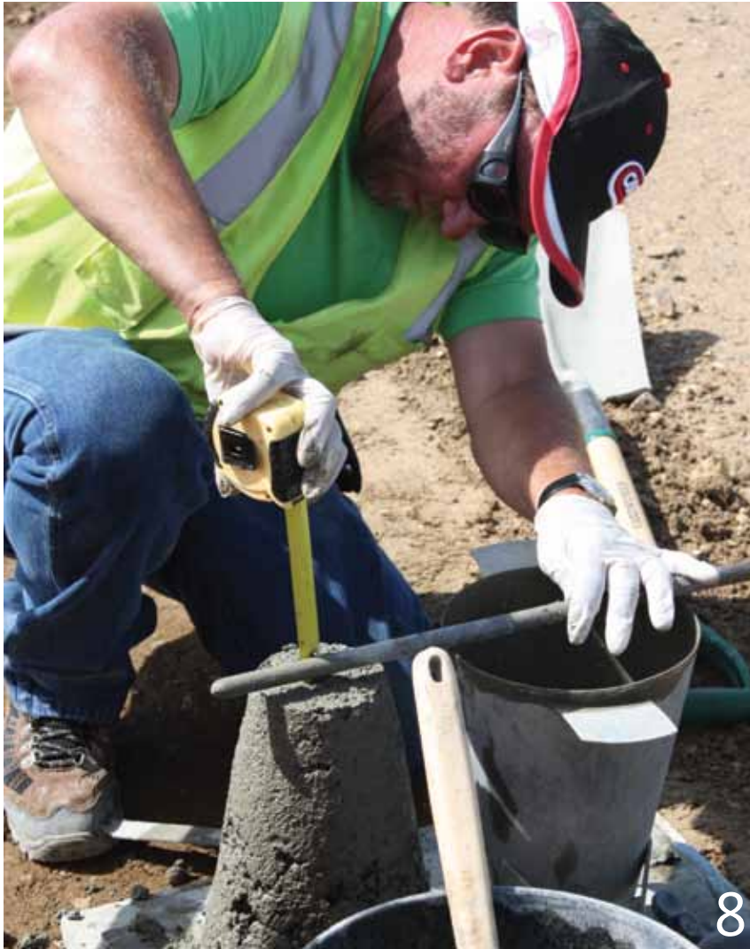
The slump test is the industry-wide standard method to measure the consistency and workability of portland cement concrete. Journey Transportation Technician Craig Orke, DOT Sioux Falls Area, takes a sample of newly placed concrete, fills the slump cone mold, rods the mold, strikes the surface flush with the tamping rod, lifts the mold vertically, measures the height difference and records the result. Slump tests are an important quality control measure.
