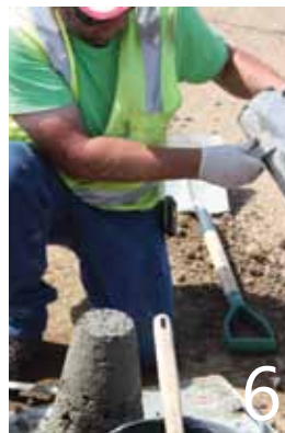
The slump test is the industry-wide standard method to measure the consistency and workability of portland cement concrete. Journey Transportation Technician Craig Orke, DOT Sioux Falls Area, takes a sample of newly placed concrete, fills the slump cone mold, rods the mold, strikes the surface flush with the tamping rod, lifts the mold vertically, measures the height difference and records the result. Slump tests are an important quality control measure.
