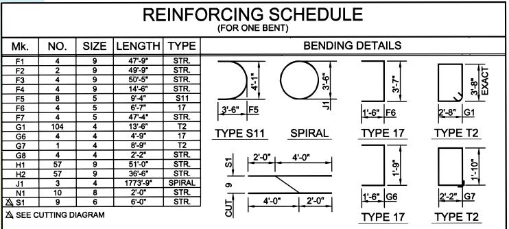
SPIRALS - USE 6" PITCH AND 1 1/2 EXTRA TURNS AT EACH END. USE 1 1/2 TURNS FOR LAP AT SPLICE AS REQUIRED, OR WELD AS APPROVED BY THE OFFICE OF BRIDGE DESIGN. USE 4 VERTICAL SPACER BARS PER COLUMN. SPIRALS MAY BE SMOOTH BARS. BAR LENGTH SHOWN DOES NOT INCLUDE SPLICES.
