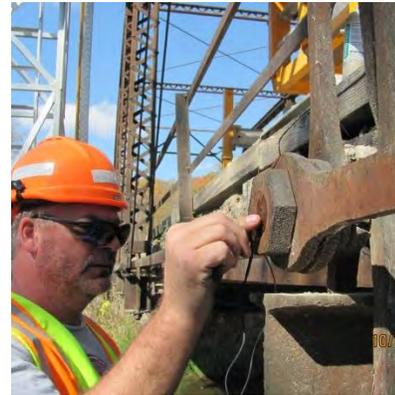
**Ultrasonic Examination of a Pinned Truss Connection**
