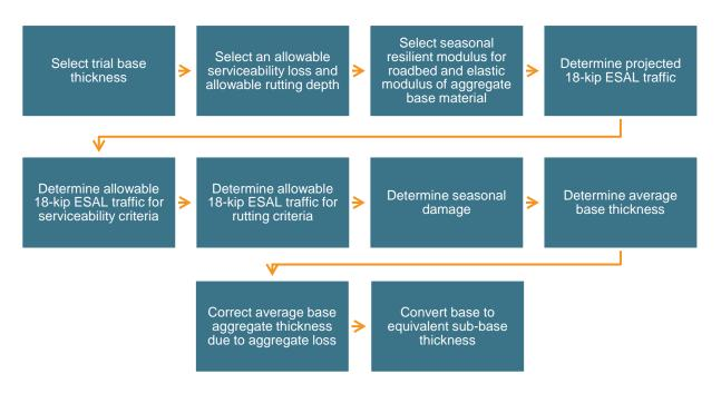
Figure 8-2: AASHTO Gravel Thickness Design Method Process
