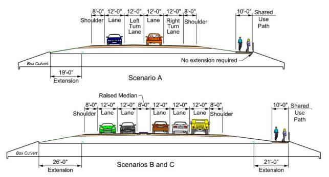
Figure 35: US14 Bypass/Western Avenue Intersection Box Culvert Typical Sections
