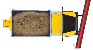
The tow plows are a 36-foot trailer, equipped with either a 250-gallon liquid deicer tank and an 8-cubic yard hopper sander, or two (2) 1,000-gallon liquid deicer tanks. The setup is decided during equipment ordering. The tow plow can deploy either to the left or the right to do a wider sweep (centerline to shoulder) of the road than a typical plow truck can make alone. The tow plows are stationed on the interstate highways and four-lane expressway roads where they can be the most efficient.
