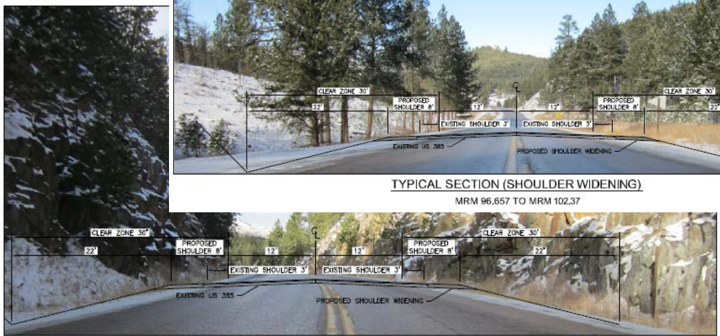
TYPICAL SECTION (SHOULDER WIDENING) MRM 87,2 TO MRM 96,657
