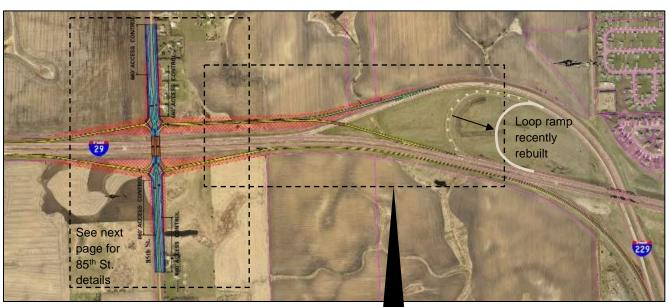
Figure 27 – Diverging Diamond Interchange (DDI) Concept Layout
