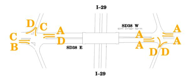
FIGURE 7 Proposed Level of Service at the Junction of SD38 and the Junction of I-29 in Sioux Falls (Exit 83) in year 2021
