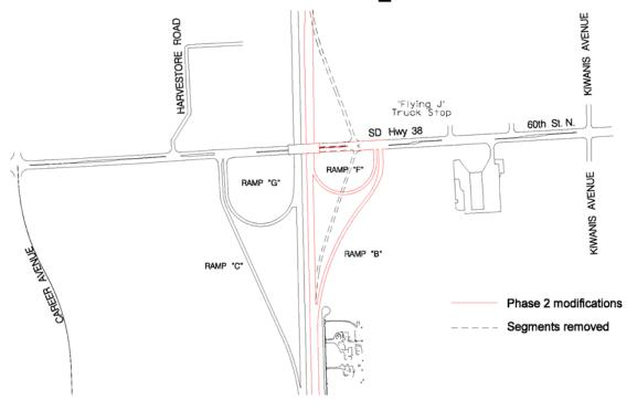
northbound on-traffic and the I-29 northbound off-ramp will relocate outside of the loop. Also, the existing Ramp A will be eliminated. Figure 9 shows the configuration of the interchange upon the completion of Phase 2. The timeframe for this reconstruction has not been set, but discussion has mentioned possibility of including with the I-90 resurfacing project scheduled for 2008 or as late as possible future reconfiguration of the I90/I29 interchange.
