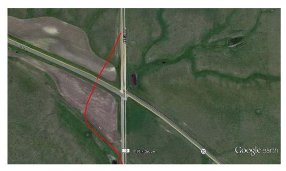
Figure 229: 448th Ave Intersection Possible Realignment Alternative
