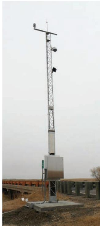
*An environmental sensor station on U.S. Highway 212 near Red Elm*
