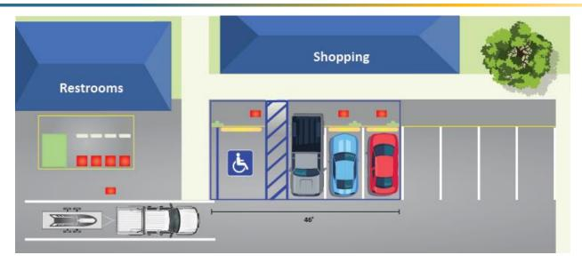
Figure 29. Potential EV DCFC Infrastructure Layout at a Travel Plaza, or Strip Mall
