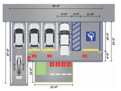
Figure 28. Basic Site Layout with Dimensions
