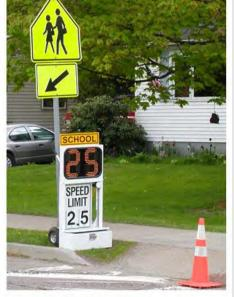
Typical portable radar speed trailer.
