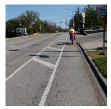
Buffered bike lane on an arterial street with no on-street parking.
