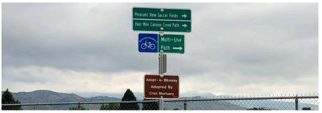
Sign assembly for intersection of independently aligned shared-use path with street NO
