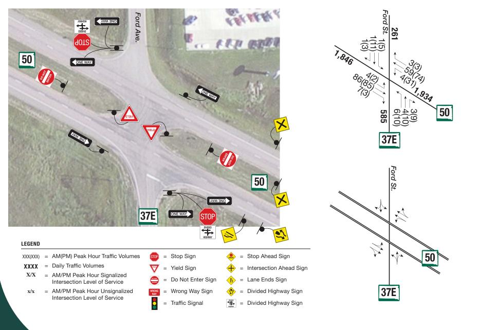
Figure 6.1 SD 50/SD 37E Traffic Conditions
