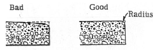
Edging will be permitted along longitudinal construction joints provided the radius does not exceed 1/4 inch. A well-defined and continuous radius shall be produced, and a smooth, dense mortar finish obtained. The surface of the slab shall not be unduly disturbed by tilting of the tool during use. **(380.3 J 7)**
