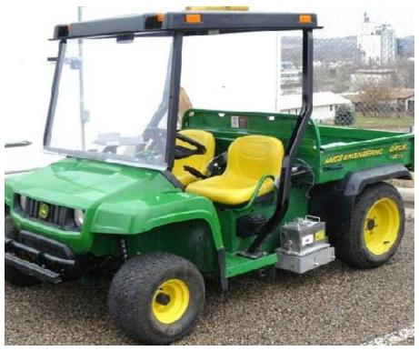
Figure 8.13 High Speed Profiler
