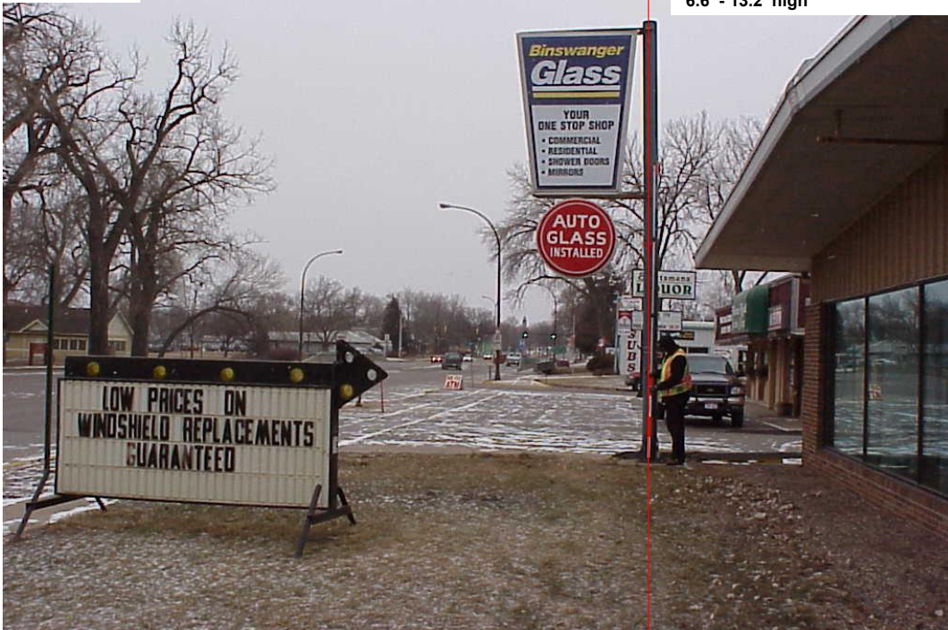
Pic. #36 (Broadway Ave.) Yankton Sta. 38+15 Lt. Binswanger Glass encroaches 6.6' - 13.2' high
