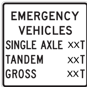
Figure 14. MUTCD R12-7aP Add-on Emergency Vehicle posting sign in current use in South Dakota. Use this sign in conjunction with another posting sign. Place EV posting sign below the other posting sign.
