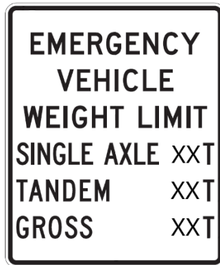
Figure 13. MUTCD R12-7 Standalone Emergency Vehicle posting sign in current use in South Dakota. Use this sign when only emergency vehicles need to be posted.
