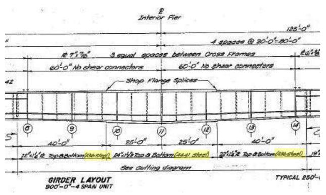
Figure 7. Details from superstructure plan sheet showing placement of A36 steel and A441 steel (highlighted in yellow) welded together into girder web.<sup>11</sup>
