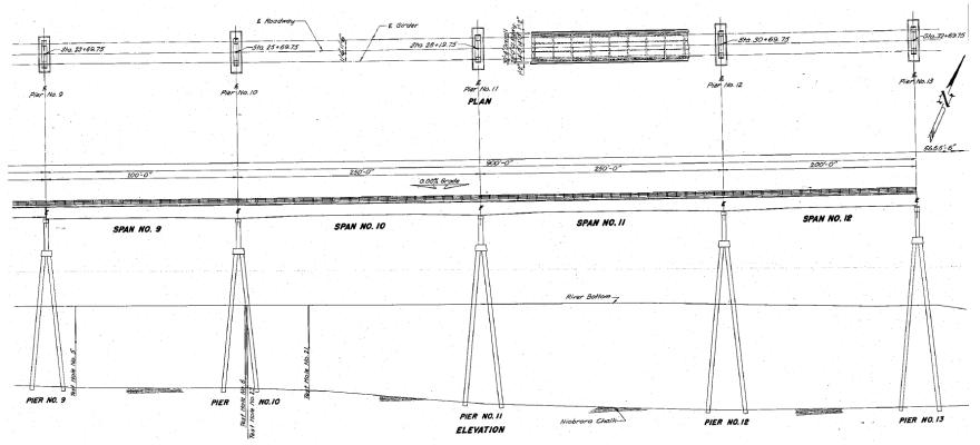
Figure 5. An example of the 900-foot four-span girder unit, shown in plan and elevation.<sup>6</sup>
