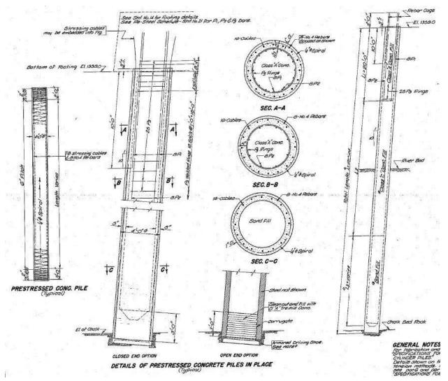
Figure 9. Details of prestressed post-tensioned concrete pile.<sup>16</sup>
