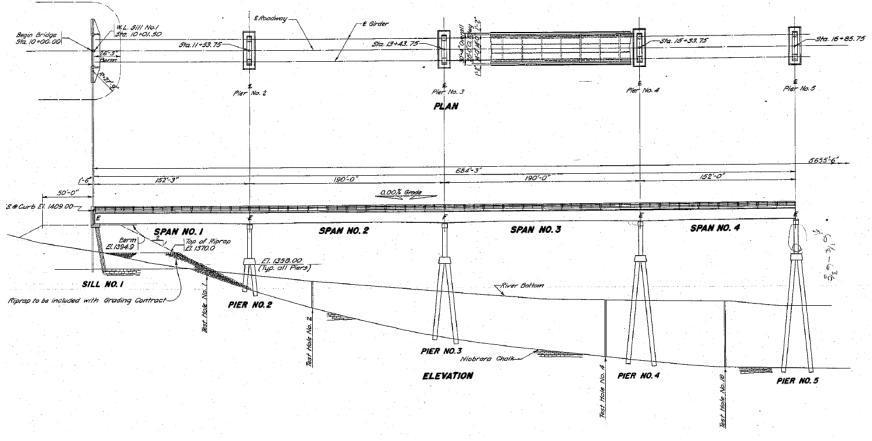
Figure 4. An example of the 684-foot, four-span girder unit, shown in plan and elevation.<sup>5</sup>
