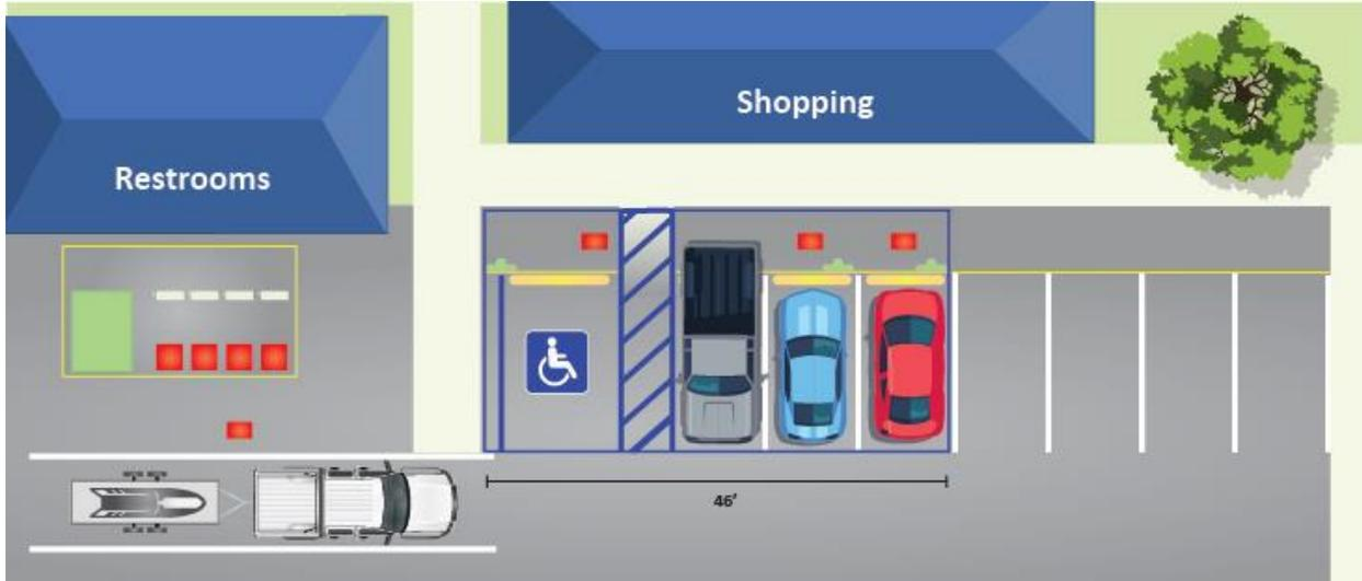
Figure 29. Potential EV DCFC Infrastructure Layout at a Travel Plaza, or Strip Mall
