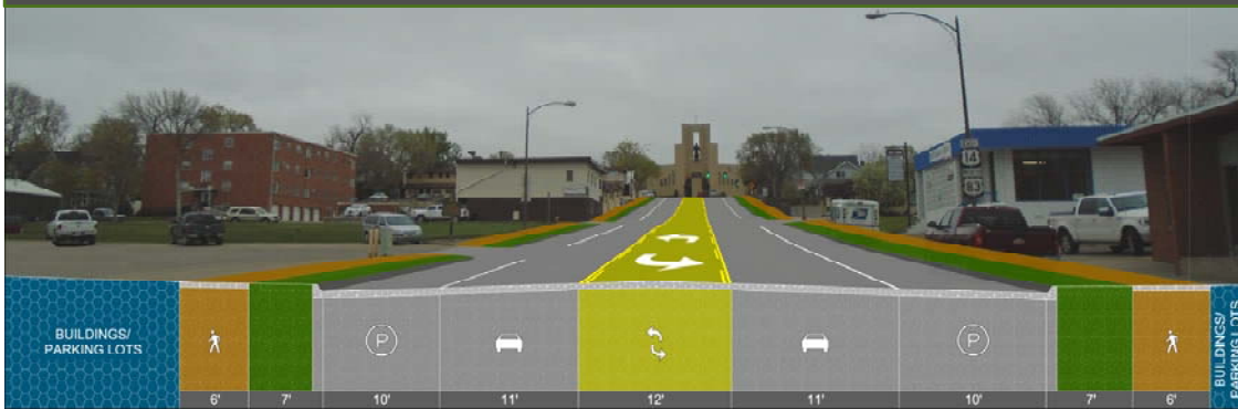
Proposed 3-lane Section - 54' Alternative 5 (40' At Intersections W/ Bulb-outs Each Side)
