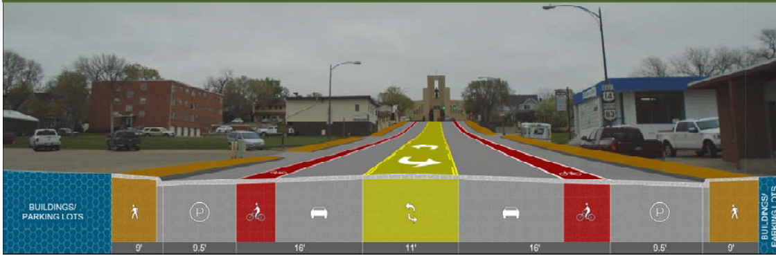
Proposed 3-lane Section - 62' Alternative 3 (50' At Intersections W/ Bulb-outs Each Side)
