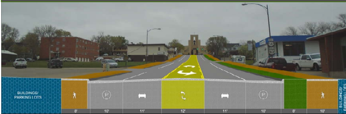
Proposed 3-lane Section - 54' Alternative 4 (40' At Intersections W/ Bulb-outs Each Side)
