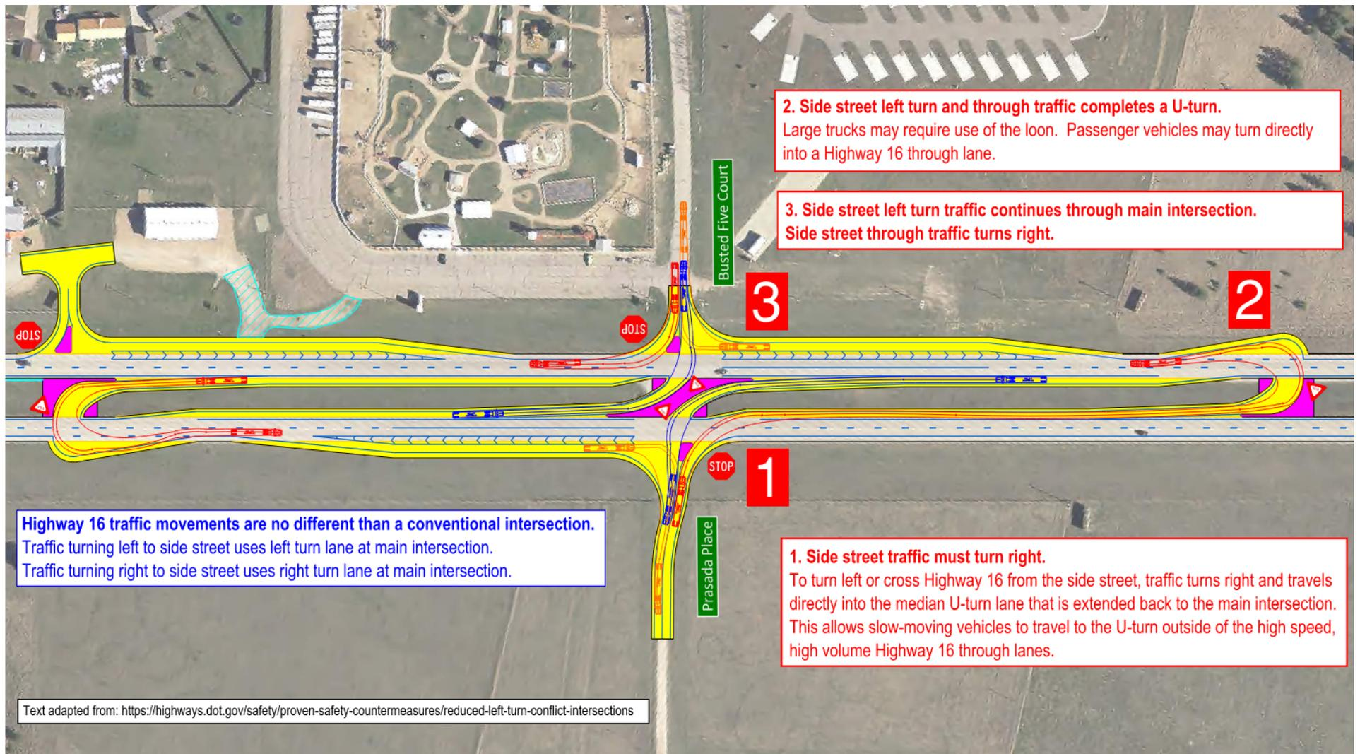
Figure 21: RCI Turn Movements - WB-67 Semi-Truck (Busted Five Court RCI, Scenario A)
