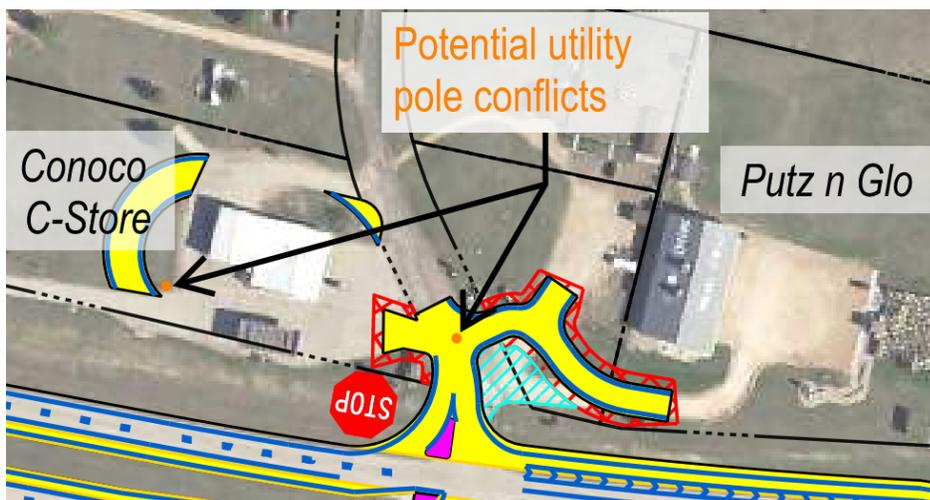
Figure 24: Scenario A C-Store Parking Modifications and Potential Overhead Power Pole Impacts
