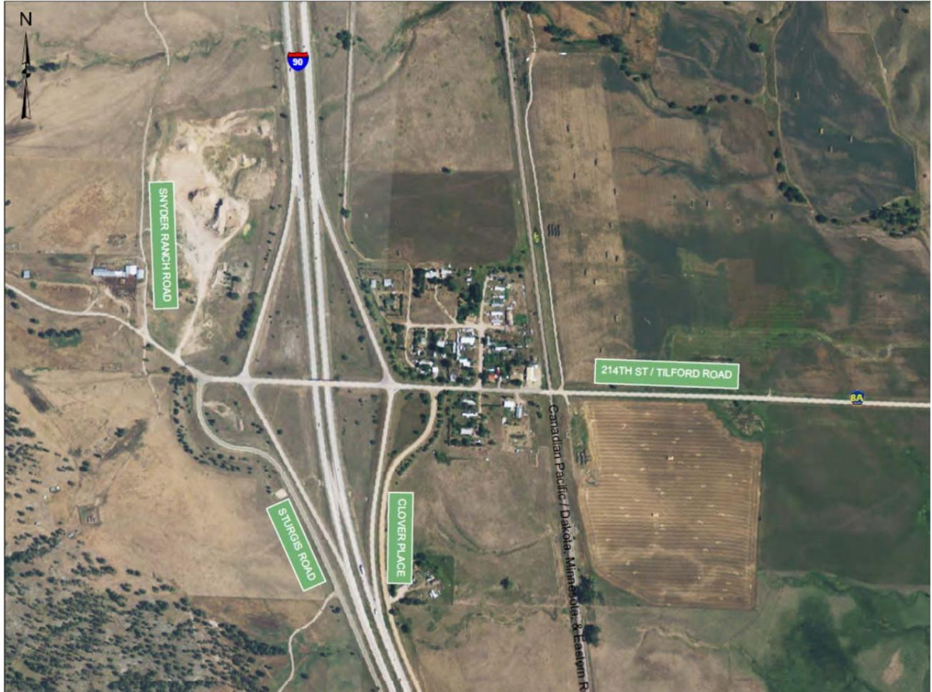
Figure 6: Existing I-90 Exit 40 Interchange Configuration
