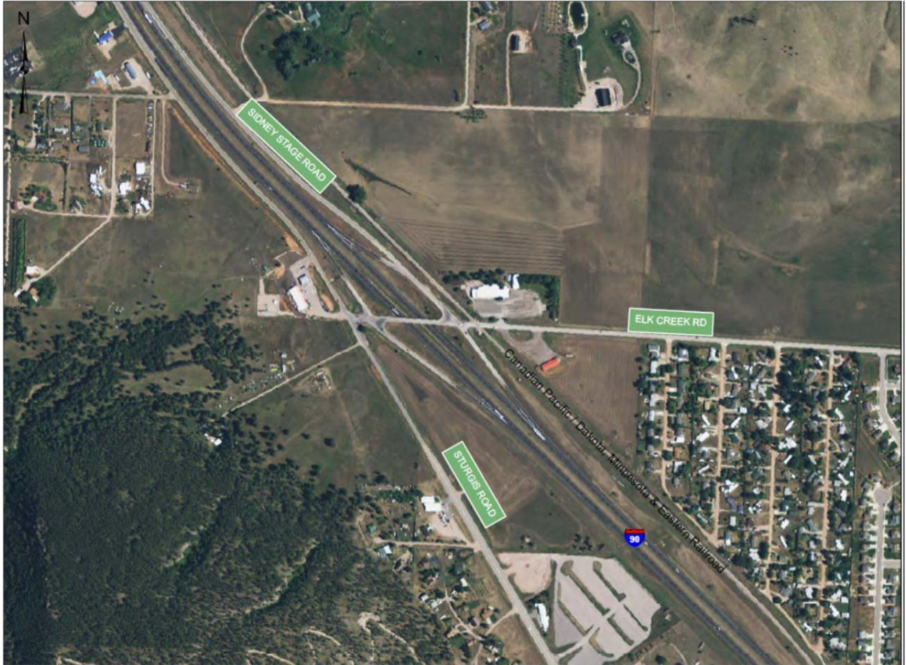
**Figure 7: Existing I-90 Exit 46 Interchange Configuration**
