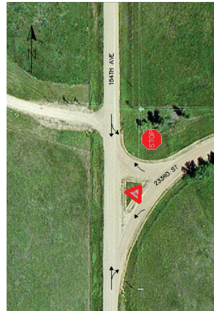
FIGURE 2 – 154 th Avenue & 233 rd Street Intersection Configuration
