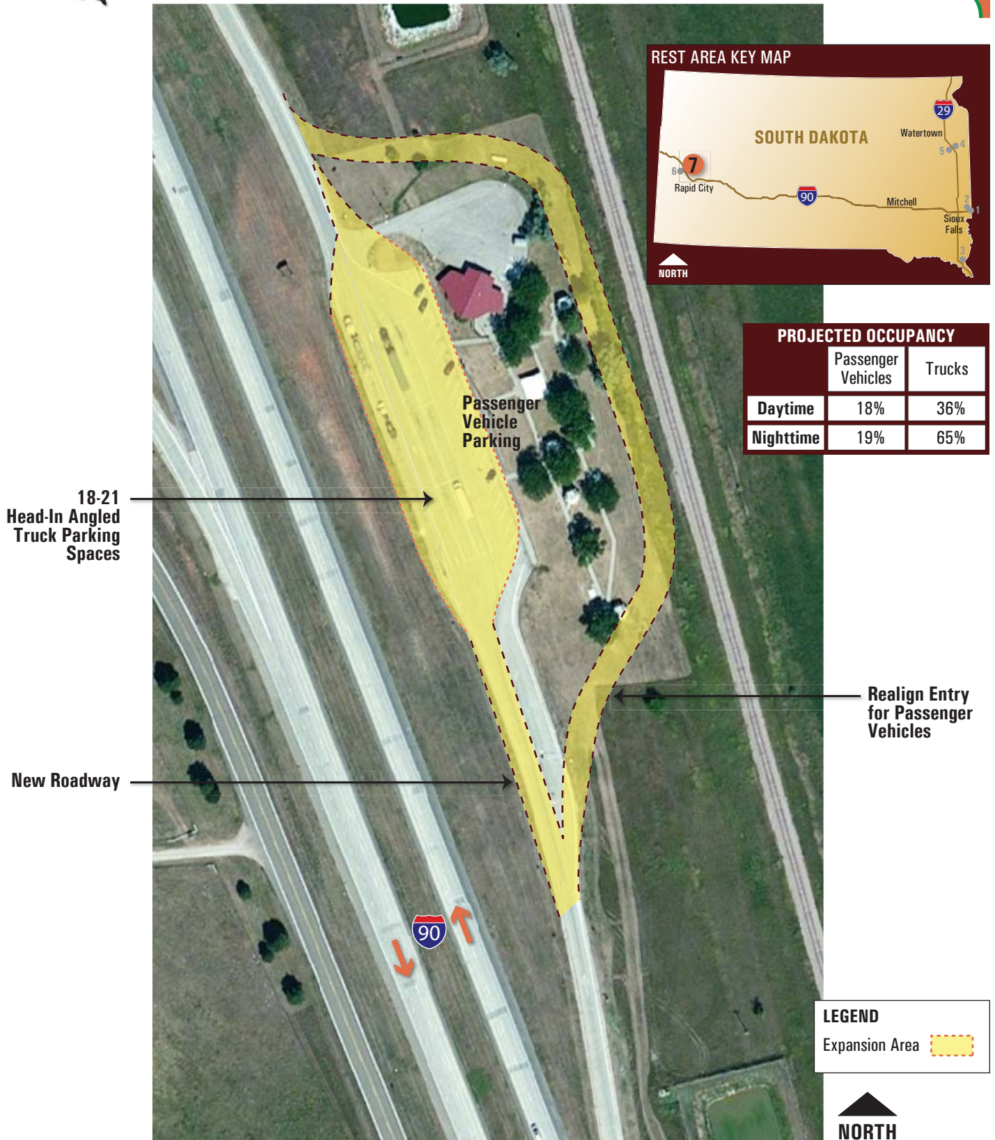
Figure 13. Tilford Westbound Rest Area Future Expansion Potential
