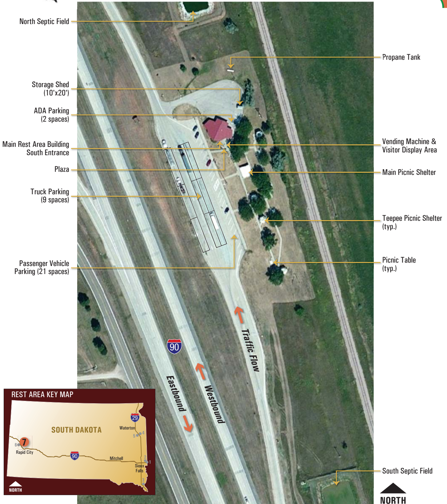
Figure 9. Tilford Westbound Rest Area Site Layout
