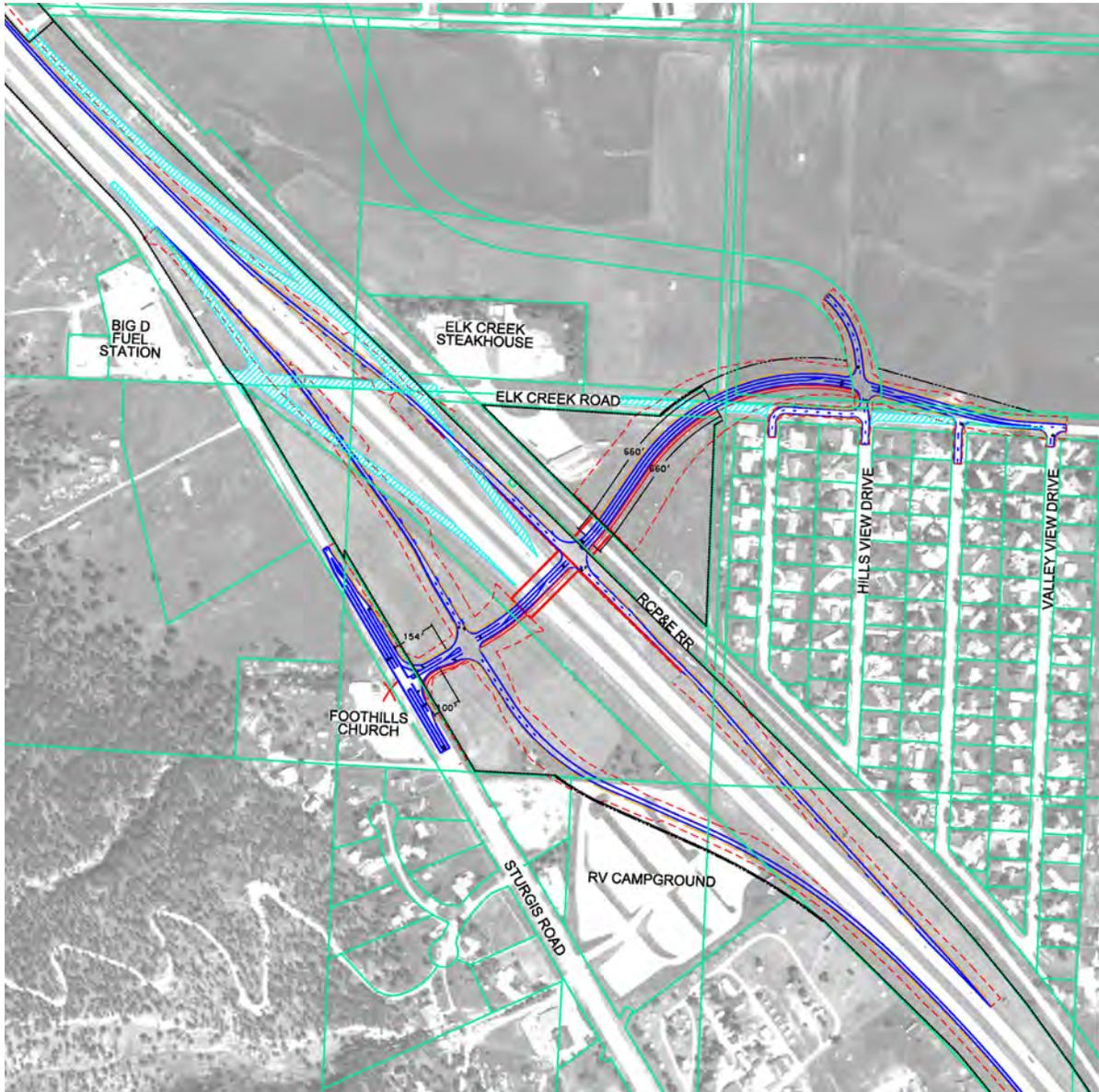
As the design of Alternative 2 progressed through development of the EA, the proposed realignment of Elk Creek Road became more pronounced to the north to allow for additional distance to accumulate height to cross the railroad and I-90 and the Elk Creek Road bridge became more perpendicular to mainline I-90. The design is further depicted on **Figures 29 and 30** in this IMJR.
