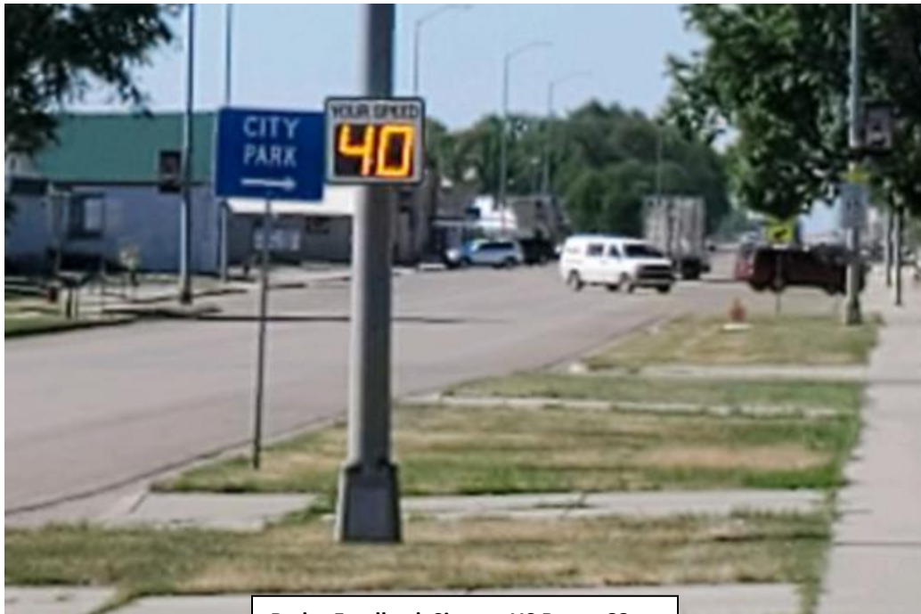
Radar Feedback Sign on US Route 83
