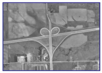
corrects the existing geometric deficiencies. The proposed full cloverleaf interchange can be constructed in phases, with the ramps for movements to and from the north added at a later date as warranted by growth and development in the area.
