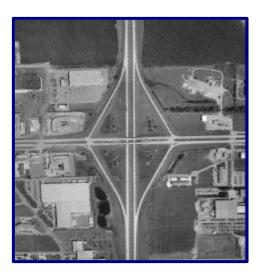
Ultimately, if traffic volumes warrant, the construction of a loop ramp in the northeast quadrant would be necessary to reduce the impact from northbound left turns and avoid a new hotel that has been constructed in the southeast quadrant. Access control along US 14 to the east and west should also be addressed at the time of improvements.
