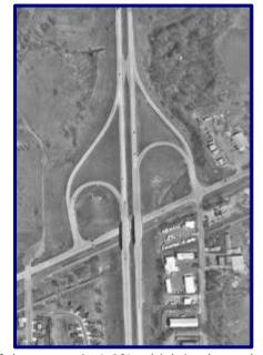
on all four of the ramps. The superelevation rate on all of the ramps is 6.0%, which is above the 4.0% criteria. The minimum horizontal radius provided on the loop ramps is only 160′, which is well below 30 mph design. The on-ramp tapers for Ramps A and H do not meet the 50:1 design criteria. The K values on the crest vertical curves for Ramps A and D are below the 50 mph design criteria, which correlates to inadequate stopping sight distances.
