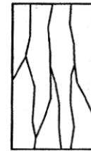
Type 3 Columnar vertical cracking through both ends, no well- formed cones
