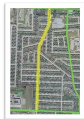
Figure 3-3: Example of Urban Minor Arterial
