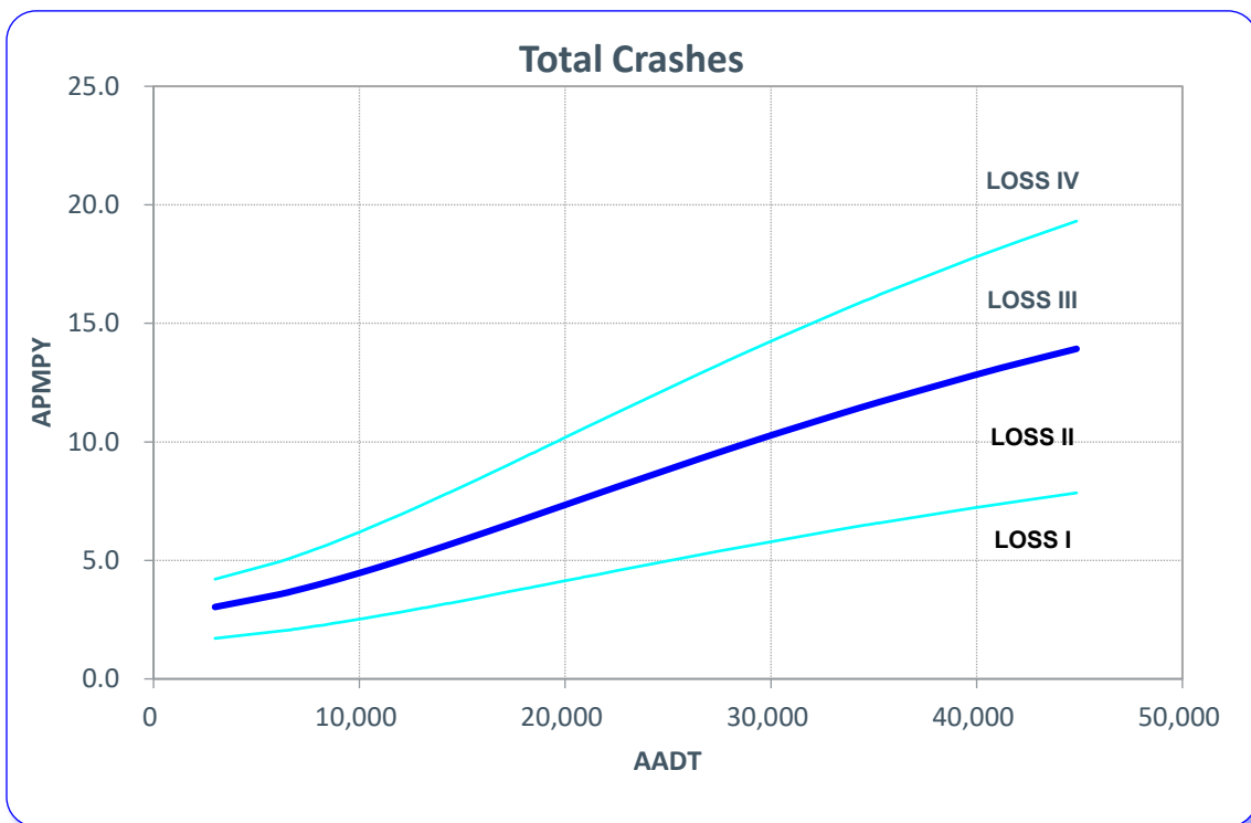
Figure 2-4. Urban 4-Lane Divided Freeway Frequency SPF
