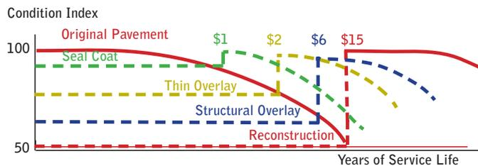
*At 50 on the condition index, pavement has zero years left of service life.*
