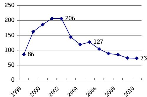
*\*In 1999, South Dakota adopted a new AASHTO rating method that caused a change in the number of structurally deficient bridges. In 2002, South Dakota adopted an AASHTO revision to the rating method that is bringing the number of structurally deficient bridges back in line with the previous trend.*
