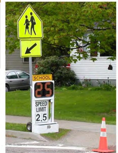
Typical portable radar speed trailer.
