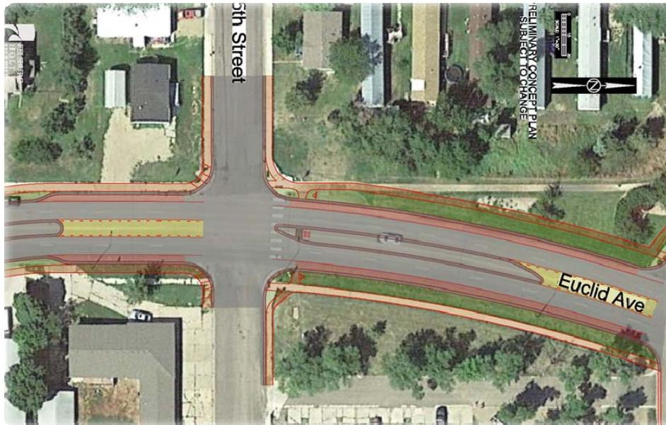
The RRFB at the intersection of US 14 (Euclid Avenue) with Fifth Street is recommended to be replaced with MUTCD compliant beacons and supplemental treatments to increase driver compliance and pedestrian safety.
