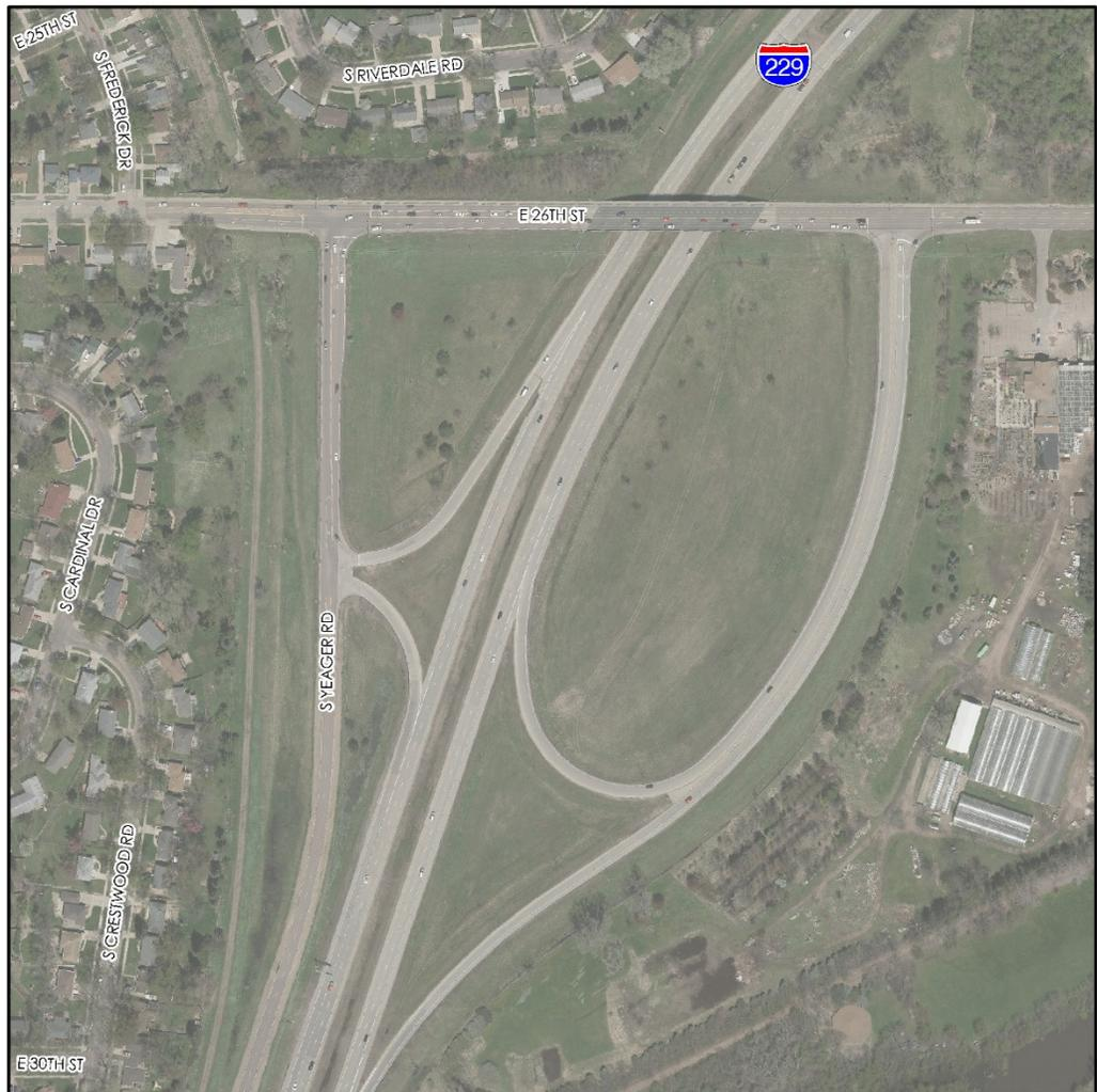
The proposed reconfiguration will reconstruct the interchange to a standard folded diamond configuration as shown in **Figure 10**. The northbound I-229 ramp connections will be widened near the ramp terminal intersection, but are unchanged near the ramp gores. The southbound ramp configuration will be entirely reconfigured.
