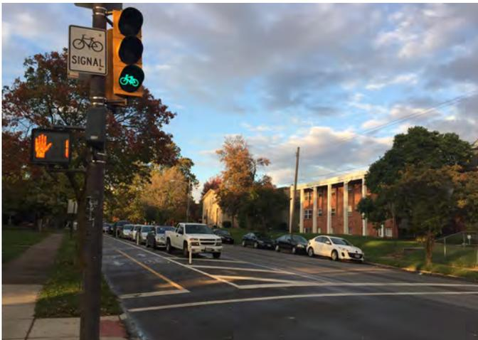
An actuated signal pavement marking (Source: NACTO)
