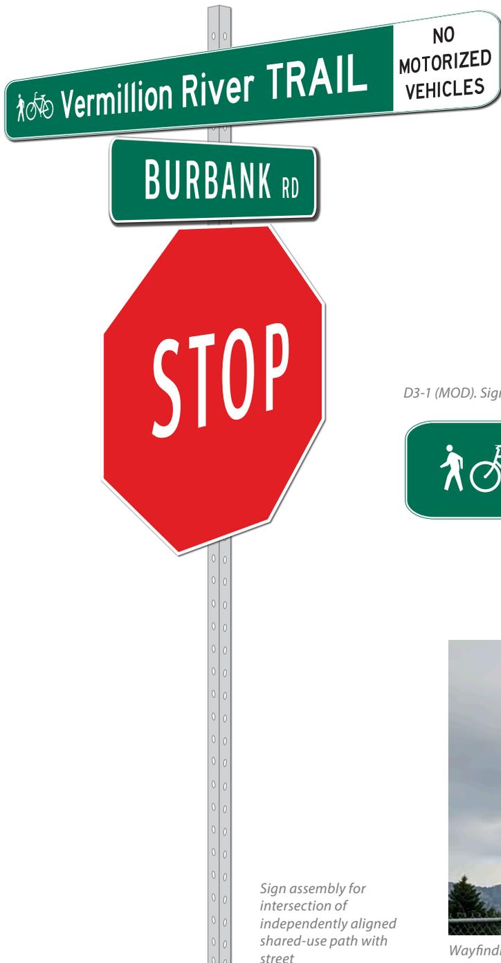
Sign assembly for intersection of independently aligned shared-use path with street
