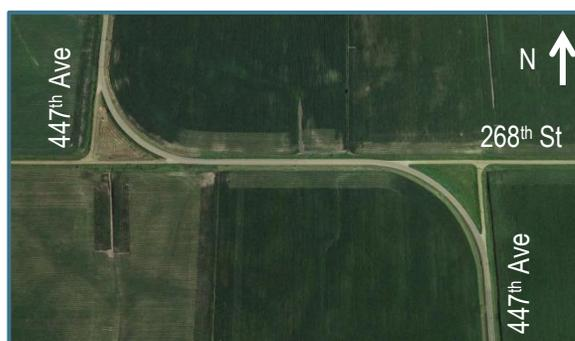
***447<sup>th</sup> Avenue horizontal curves through section line correction at 268<sup>th</sup> Street.***
