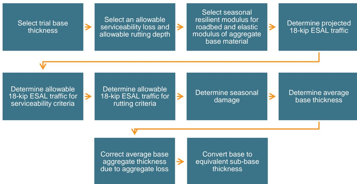
**Figure 8-2: AASHTO Gravel Thickness Design Method Process**
