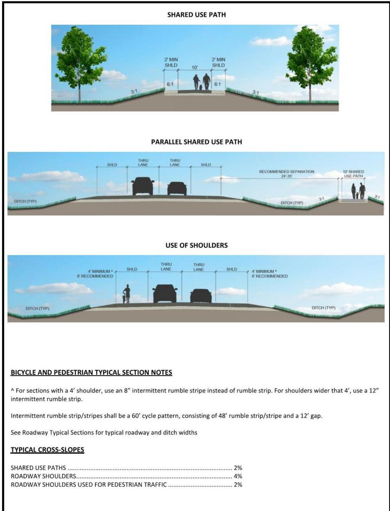
Figure 8-3: Typical Multi-Modal Facility Cross-Sections
