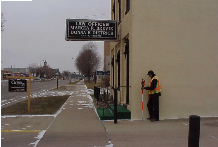
Pic. #51 (Broadway Ave.) Yankton Sta. 19+80 Lt. Law Offices encroaches 1.2'
