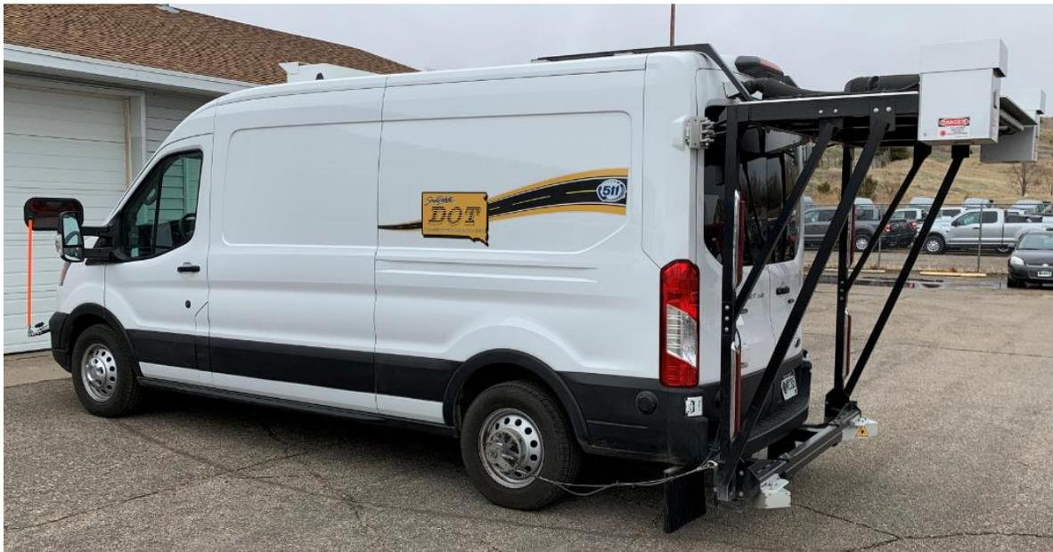
*Figure 3.8: Road and Pavement Data Collection Vehicle*
