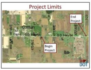
**Background Information** Structure in 1963 Grading & Interim Surfacing in 1984 PCC Surfacing in 1985 Low Slump Dense Concrete (LSDC) Overlay in 1997 Dowel Bar Retrofit and Pavement Repair in 2004 Joint and Spall repair in 2018
