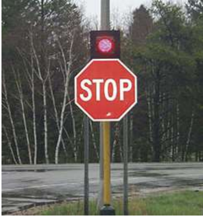
Figure 1a. Stop Sign with Stop Beacon
