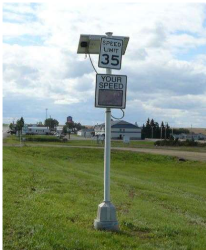
Figure 4. RSFS with Speed Limit sign installed in Selby, SD
