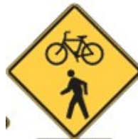
Figure 7c. Trail Crossing Warning Sign (W11-15)
