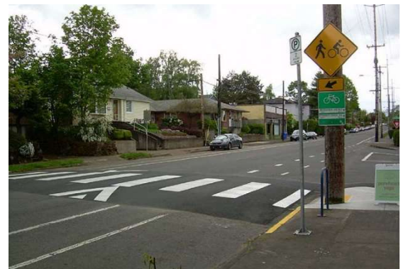
Figure 14. Raised Pedestrian Crossing
